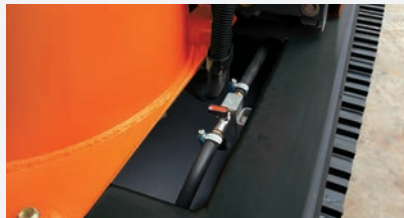
Fuel tank water drainage cock
