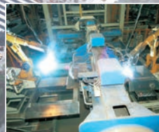
Main frame welding line
