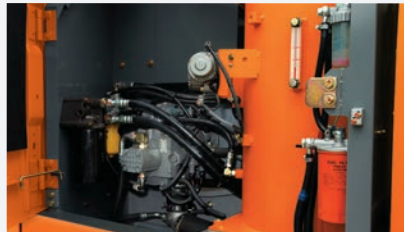
Grouped remote filters and inspection points
